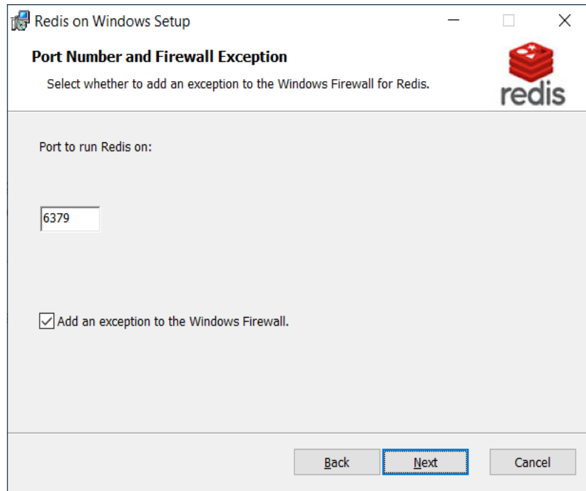
Figure 38. Redis Setup – Port Number and Firewall Exception Configuration
